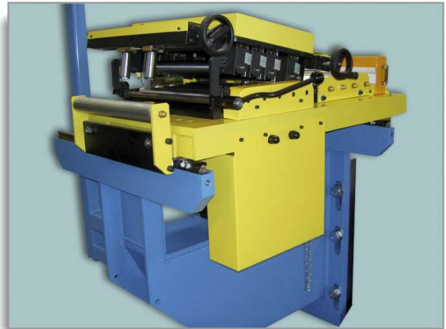
Detailed view of opened head with central edge guides and heavy-duty bracket for press-mounting. The zigzag motion allows maximum usage of strip surface through staggered stamping
