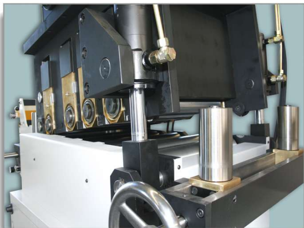
Heavy Straightener-Feeder w opened alligator head: With sturdy design like this our engineering allows even most strenuous jobs to be handled with confidence
