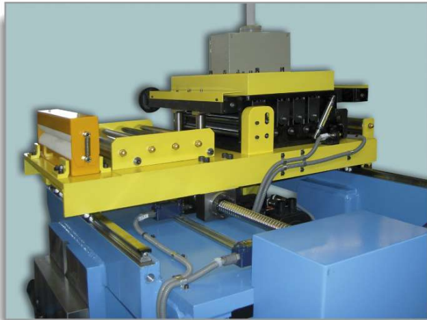
Straightener-Feeder with zigzag option and lubricator. Lateral motion on servo-driven spindle; body guided on precision linear bearings
