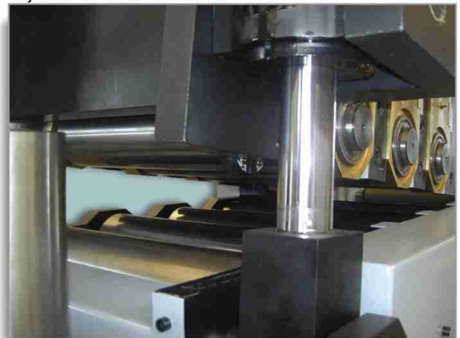
Opened alligator head - the wide gap demonstrates how easily the inside can be accessed for threading, cleaning or maintenance purposes
