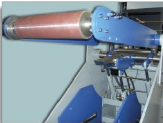
Detail on threading system with pre-bending roll and peeler wedge. Hydraulic hold-down arm with powered, polyurethane covered roller.
