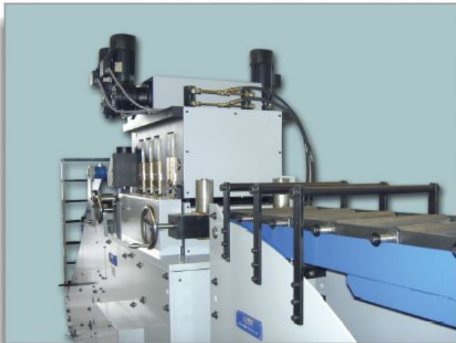
Heavy 400 mm wide Cradle-Straightener for over 10 mm materials. With motorized straightening roller adjustment and clock-spring guard.
