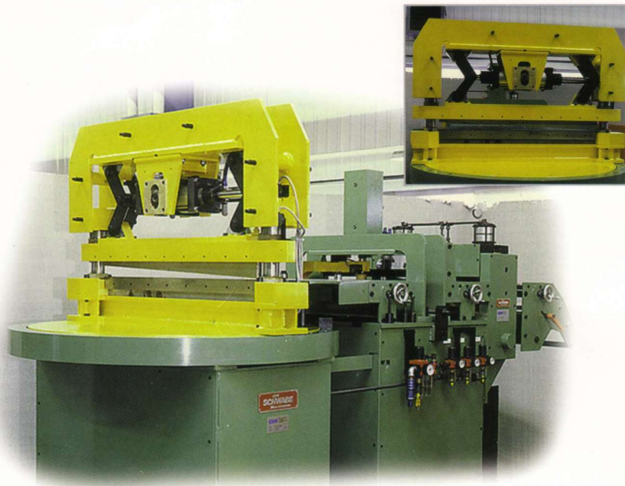
Special shears in a production line for laminated material
